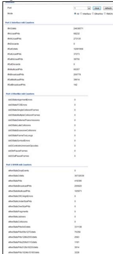
Figure 34 Monitor > Port > Port > Port Counters
